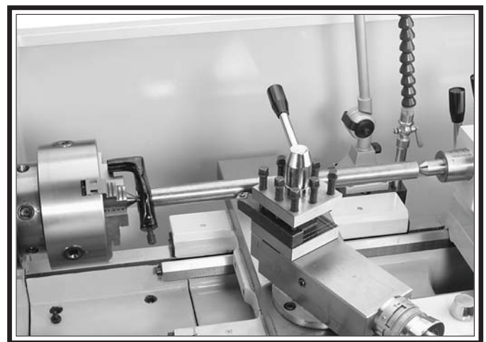
Figure 54. Example photo of a workpiece mounted between the centers.
